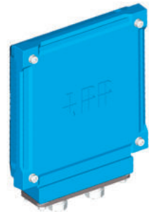
Auxiliary cast iron terminal box (variant code 567). 208 x 180 mm, max 30 strips. Earthing M6
